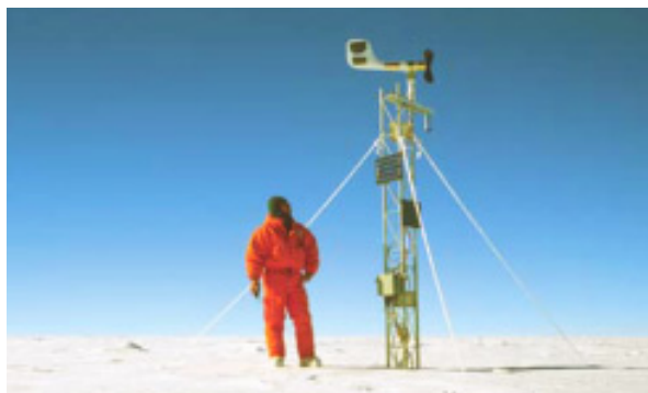
Slika 2. Samodejna meteorološka postaja na Antarktiki Figure 2. An automatic weather station in the Antarctic
