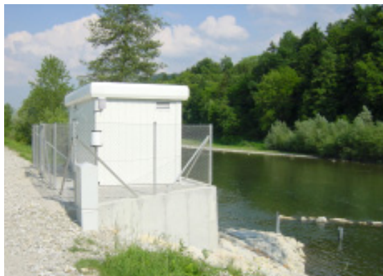
Slika 3. Samodejna merilna postaja za spremljanje kakovosti površinske vode na Savinji v Medlogu Figure 3. Automatic measuring station for surface water quality monitoring at Savinja in Medlog
